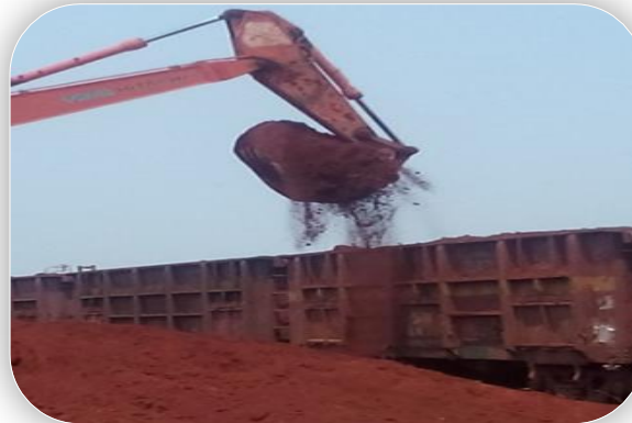
LOADING RED MUD IN RAIL WAGONS
